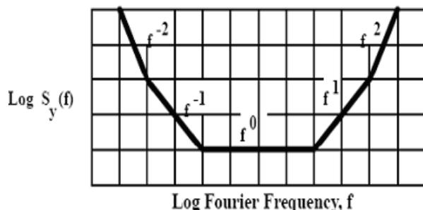
Time domain frequency stability measure (Allan Deviation) is related to the spectral density of the fractional frequency fluctuations by the relationship given below [8]:
