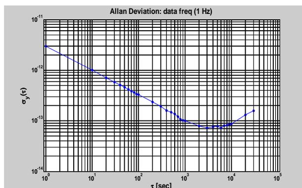
Figure 4: Allan deviation of a rubidium clock
