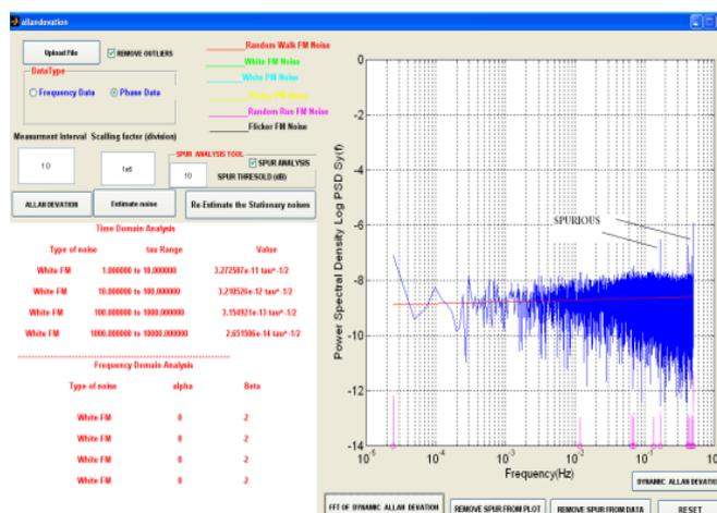
Figure 9: Spurious profile of Rubidium clock data
