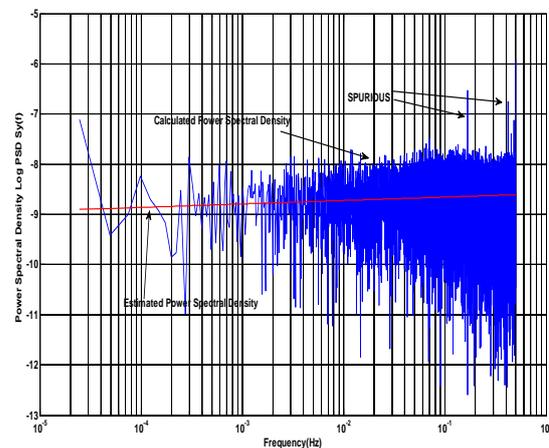
Figure 7: Spurious profile for rubidium clock data
