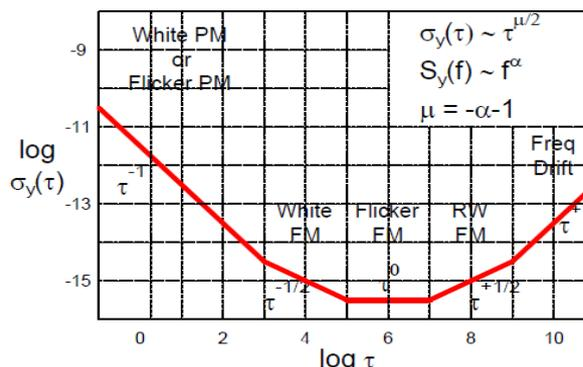
Figure 2: Allan Deviation ( $\sigma_y(t)$ ) of the Clock Noise Error Sources [9]
