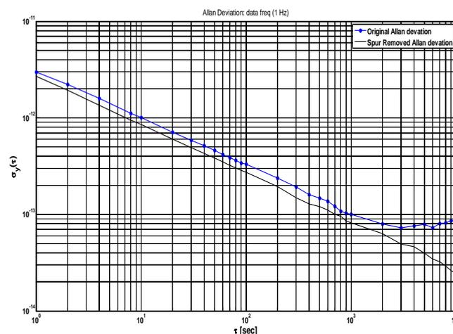
Figure 10: Comparative stability plot of Rubidium clock data<sup>2</sup>
