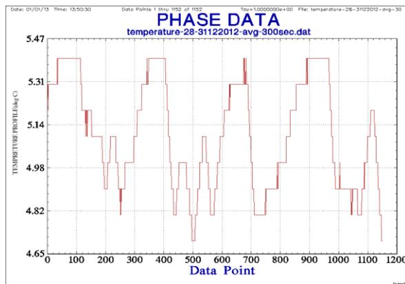
Figure 5: Temperature variation profile of rubidium clock
